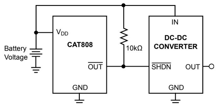
**Note:** The value of the pull-up resistor is not critical
