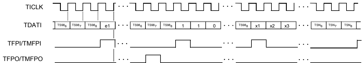
Figure 69 Framer Mode J2 Transmit Input Stream
