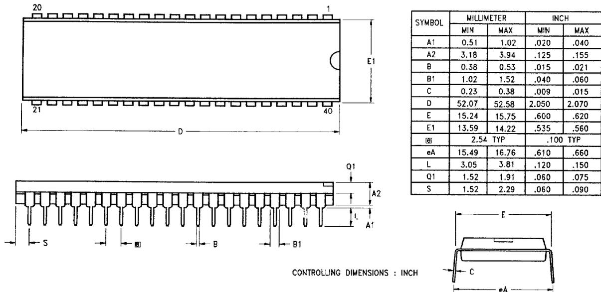
Figure 62. 40-Pin DIP Package Diagram
