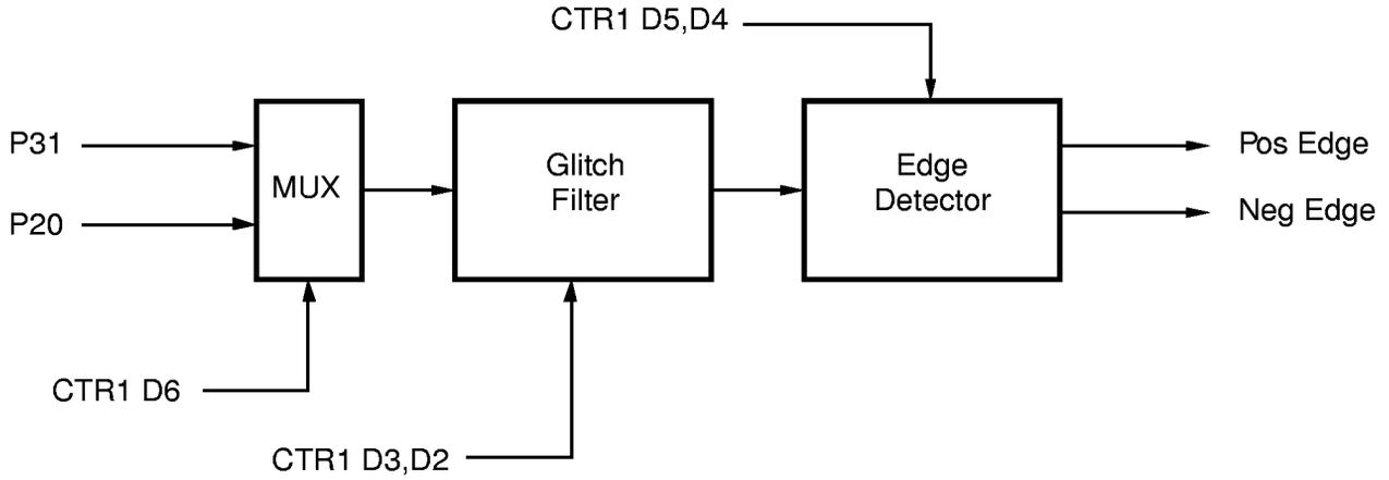
**Figure 22. Glitch Filter Circuitry**
