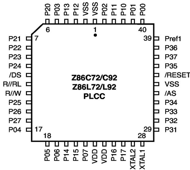
**Figure 4. 44-Pin PLCC Pin Assignments**
