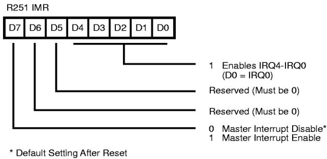
**Figure 57. Interrupt Mask Register**
