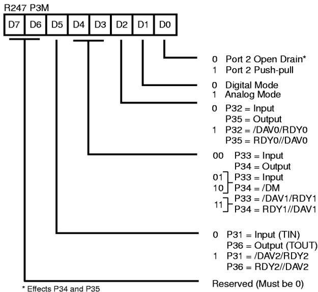
Figure 52. Port 3 Mode Register (F7H: Write Only)
