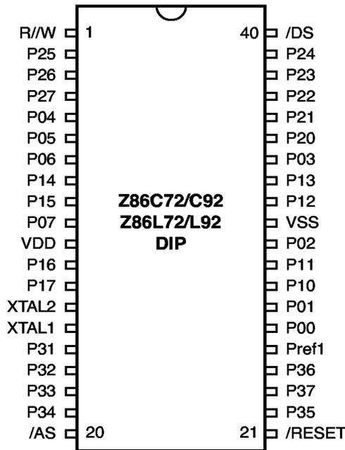
**Figure 3. 40-Pin DIP Pin Assignments**
