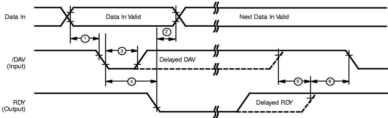
**Figure 9. Port I/O with Input Handshake Timing**
