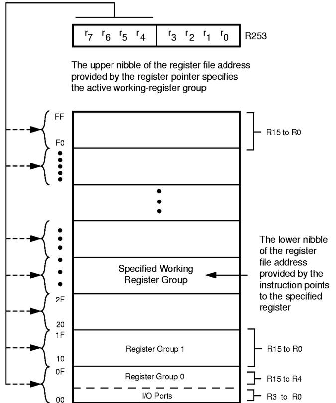
Figure 21. Register Pointer
