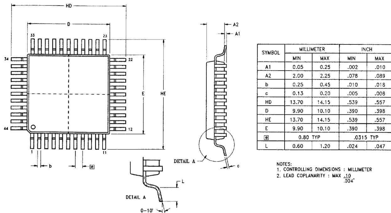
Figure 64. 44-Pin QFP Package Diagram
