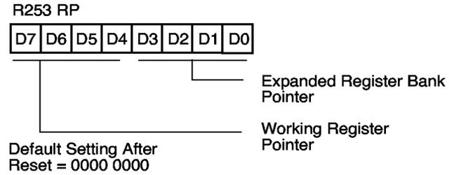
**Figure 59. Register Pointer**
