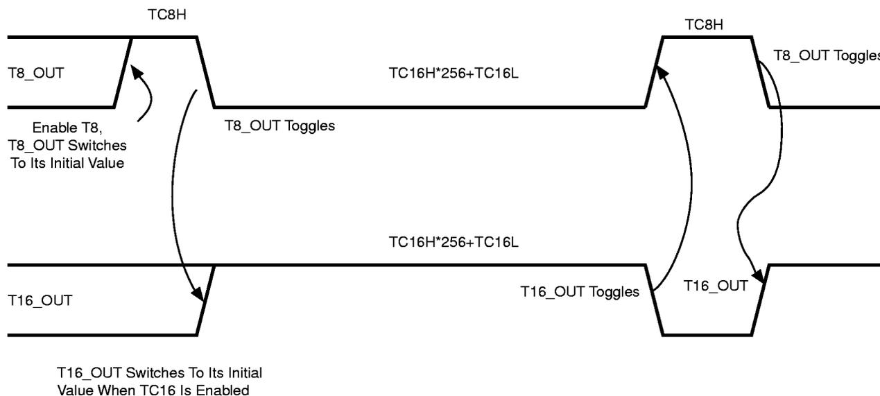
**Figure 33. T8\_OUT and T16\_OUT in Ping-Pong Mode**
