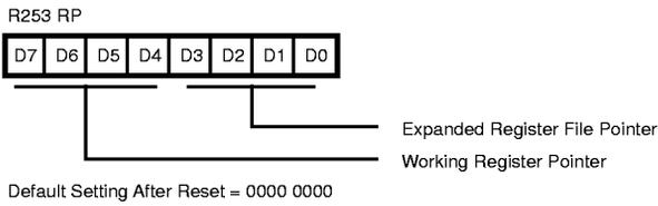
Figure 20. Register Pointer
