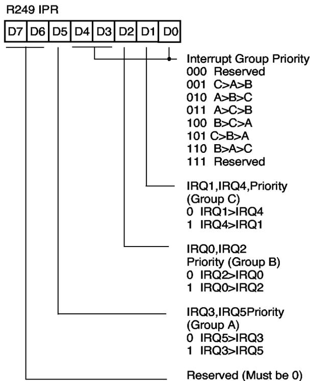
Figure 55. Interrupt Priority Register ((0) F9H: Write Only)
