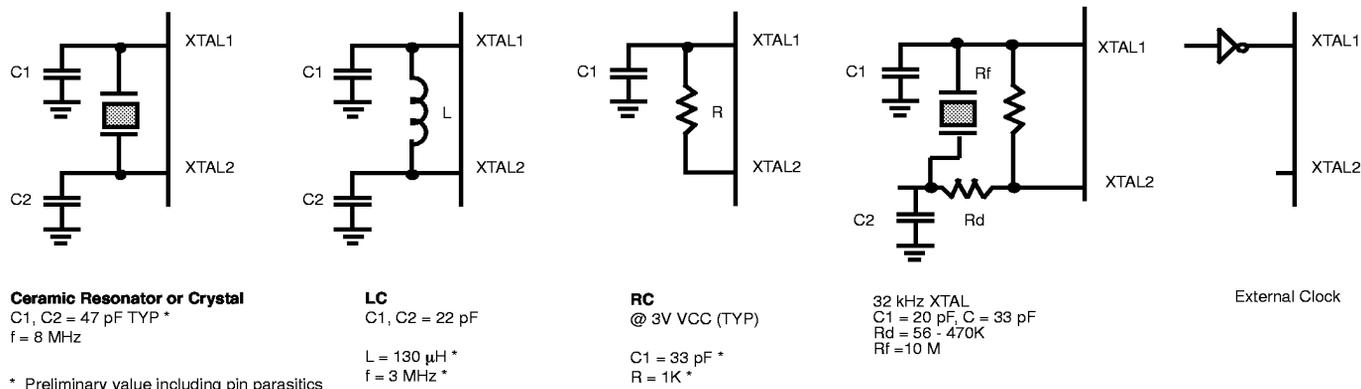
Figure 36. Oscillator Configuration
