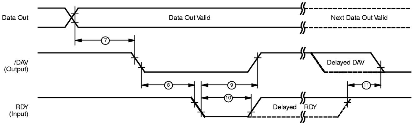
**Figure 10. Port I/O with Output Handshake Timing**
