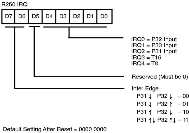
**Figure 56. Interrupt Request Register**
