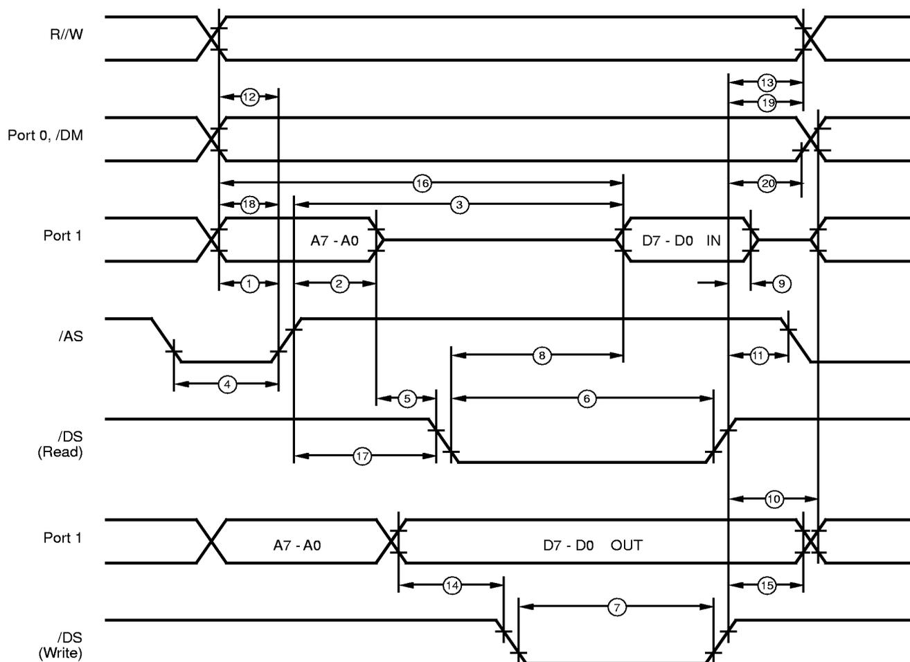
**Figure 7. External I/O or Memory Read/Write Timing**
