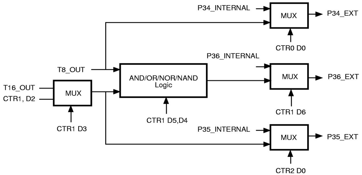
Figure 34. Output Circuit
