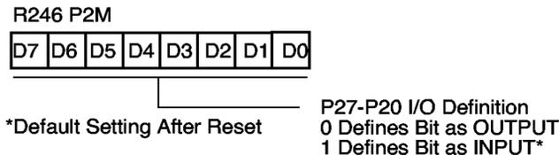
Figure 54. Port 2 Mode Register (F6H: Write Only)
