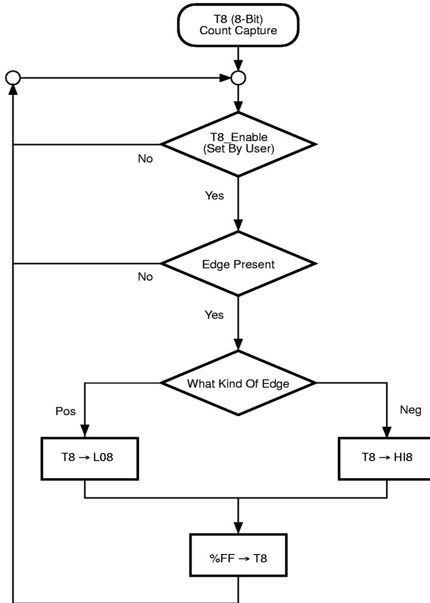
**Figure 26. Demodulation Mode Count Capture Flowchart**
