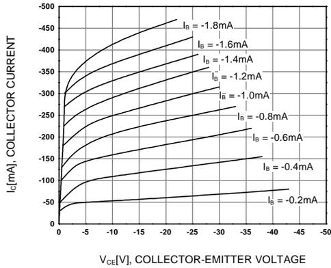
Figure 1. Static Characteristic
