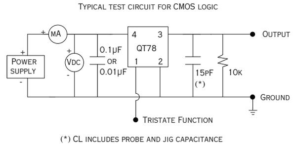
The Trisate function on pin 1 has a built-in pull-up resistor typical 50kΩ, so it can be left floating or tied to Vdd without deteriorating the electrical performance.
