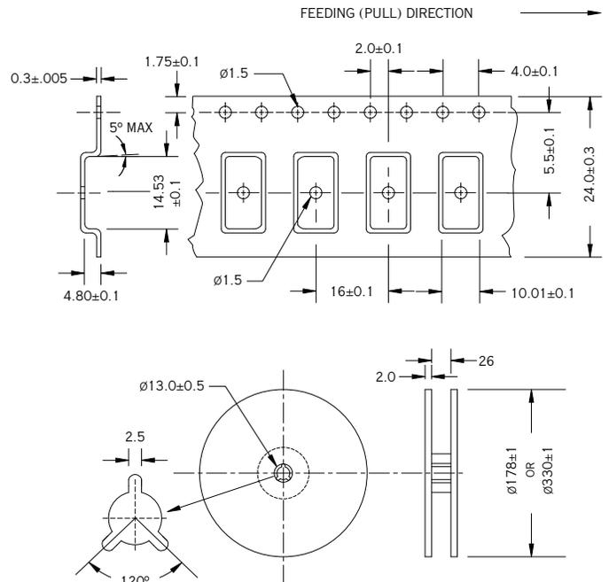
Dimensions are in mm. Tape is compliant to EIA-481-A.
