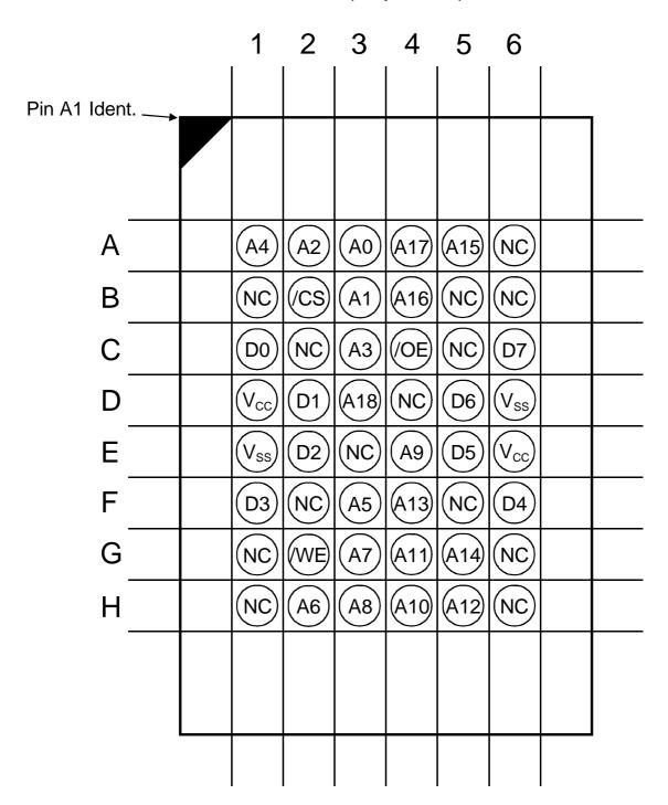
Note: Pinout shows top view, balls facing down.
