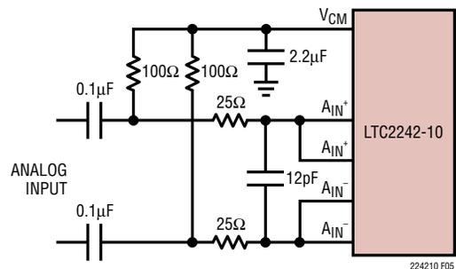
Figure 5. Capacitively-Coupled Drive
