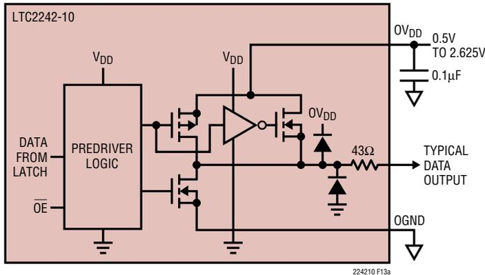
Figure 13a. Digital Output Buffer in CMOS Mode
