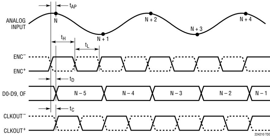
**Full-Rate CMOS Output Mode Timing**
