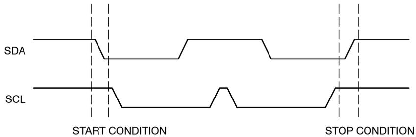
Figure 4. Start/Stop Timing
