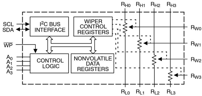
**Figure 1. Functional Diagram**
