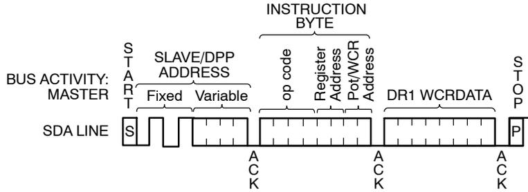
Figure 7. Write Timing
