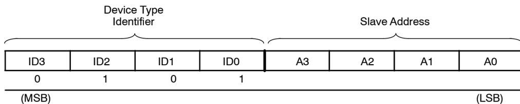
Figure 8. Identification Byte Format
