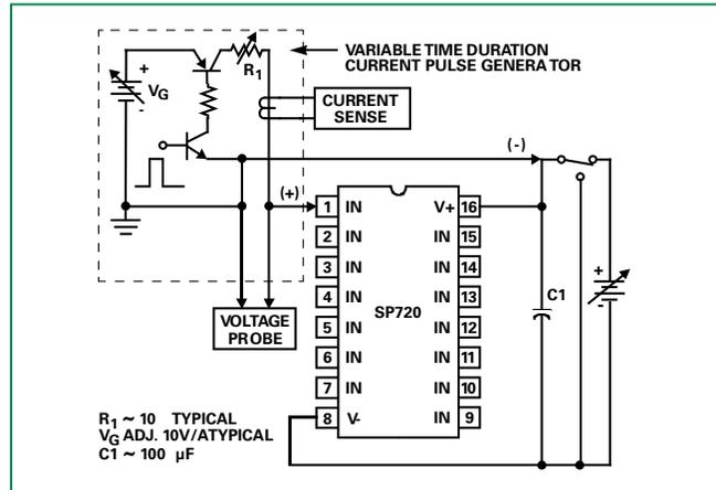
**Figure 5: SP720 Typical Nonrepetitive Peak Current Pulse Capability**
