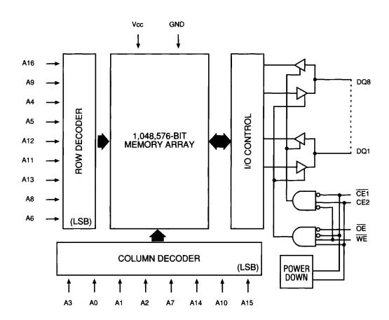
NOTE: The two least significant row address bits (A8 and A6) are encoded using a gray code.
