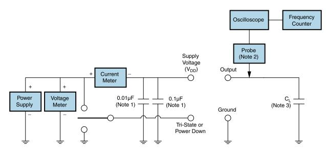
Note 1: An external 0.01µF ceramic bypass capacitor in parallel with a 0.1µF high frequency ceramic bypass capacitor close (less than 2mm) to the package ground and supply voltage pin is required. Note 2: A low input capacitance (<12pF), 10X Attentuation Factor, High Impedance (>10Mohms), and High bandwidth (>300MHz) passive probe is recommended.
