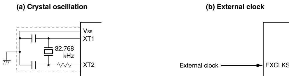
Figure 6-10. Example of External Circuit of XT1 Oscillator
