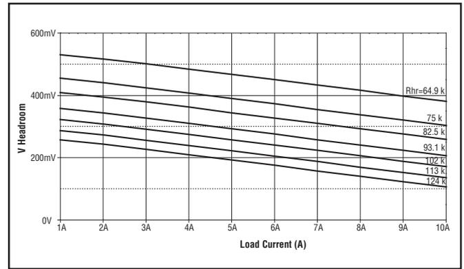
Figure 8 - Effect of slope adjust on headroom value with increasing current and RSA = 8.2 k.
