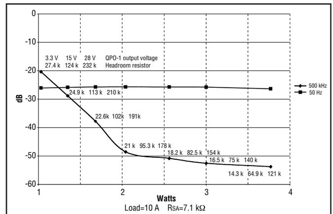
Figure 10 - Attenuation vs. power dissipation with slope adjust.
