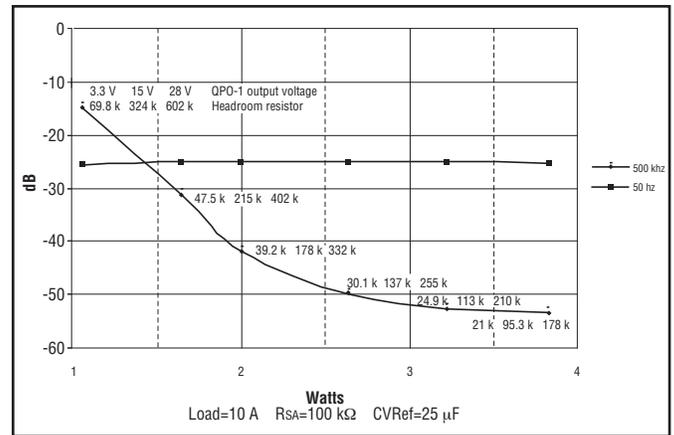
Figure 9 - Attenuation vs. power dissipation without slope adjust.
