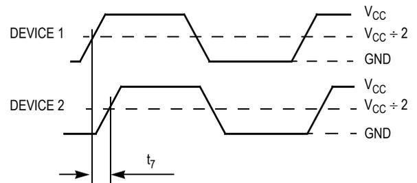
Figure 4. Device-to-Device Skew
