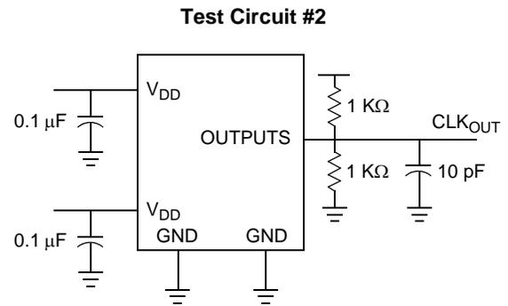
Test Circuit for  $t_8$ , Output slew rate on -1H, -5 device**Ordering Information (Available)**
