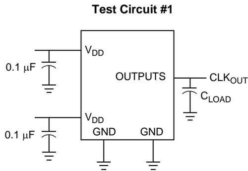
Test Circuit for all parameters except  $t_8$
