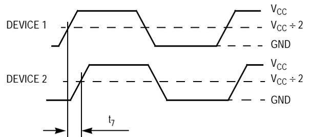
Figure 4. Device-to-Device Skew
