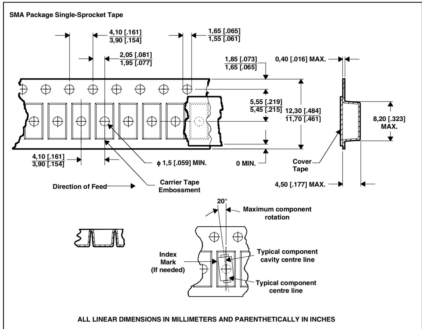
NOTES: A. The clearance between the component and the cavity must be within 0,05 mm (.002 in) MIN. to 0,65 mm (.026 in) MAX. so that the component cannot rotate more than 20° within the determined cavity. MDXXCGA
