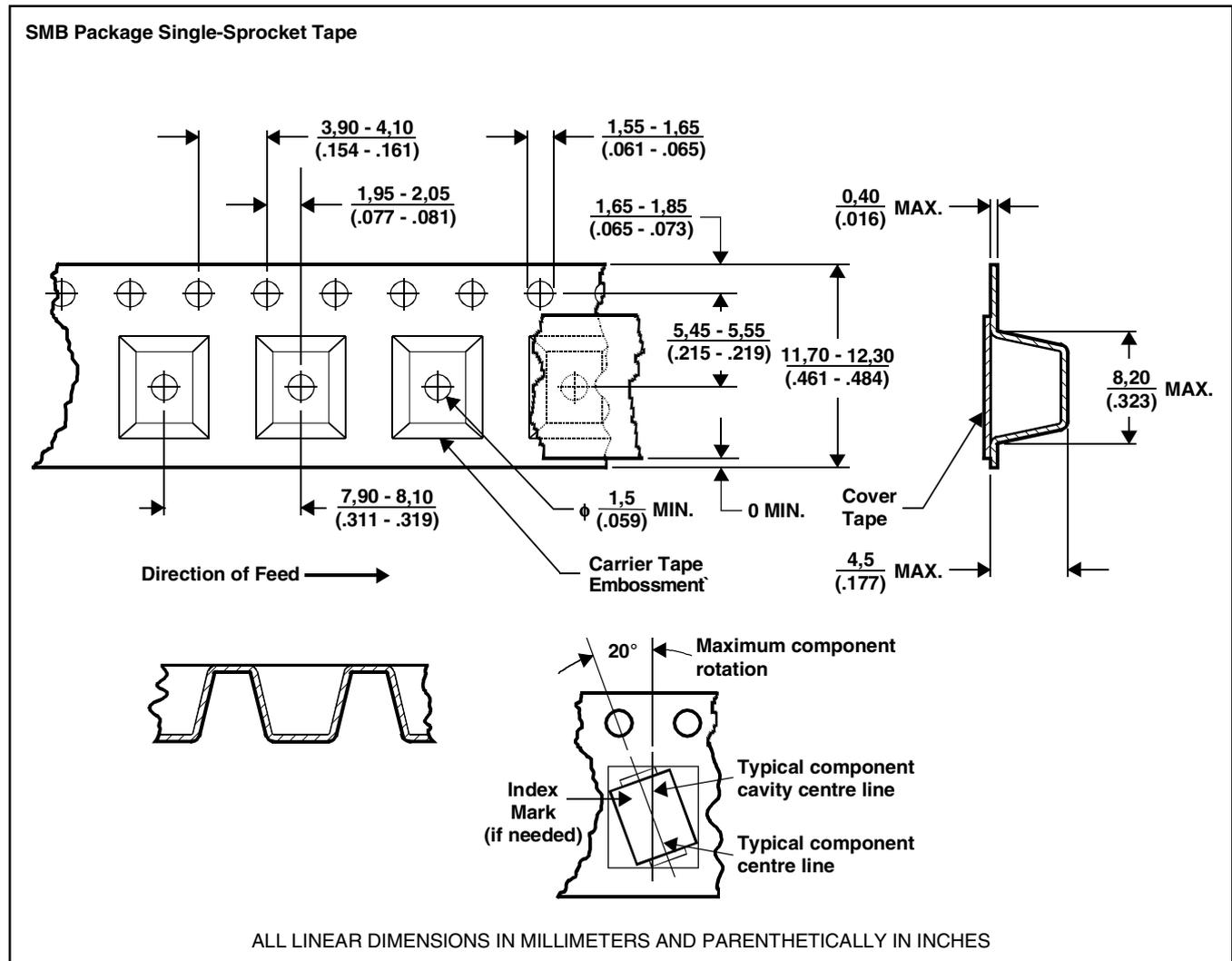
NOTES: A. The clearance between the component and the cavity must be within 0,05 mm (.002 in) MIN. to 0,65 mm (.026 in) MAX. so that the component cannot rotate more than 20° within the determined cavity. MDXXBJA
