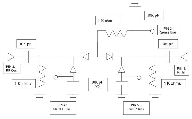
Note: Keeping PIN 4 & PIN 5 as Separate Bias Points (Same V) reduces RF leakage (increases attenuation) through an otherwise connected Common Anode Bias Node.
