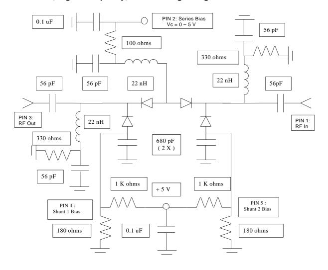
Note : Keeping PIN 4 & PIN 5 as Separate Bias Points ( Same  $\,$  V ) reduces RF leakage through an otherwise connected Common Anode Bias Node.
