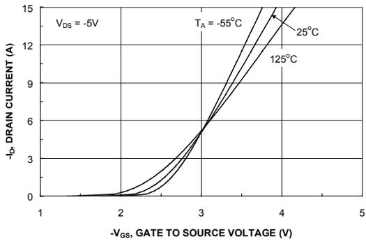
Figure 5. Transfer Characteristics.
