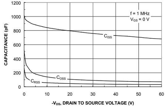
Figure 8. Capacitance Characteristics.
