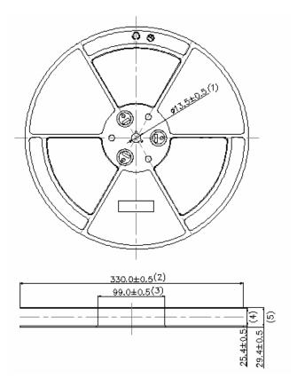
Note: 1. Dimensions are in millimeters
