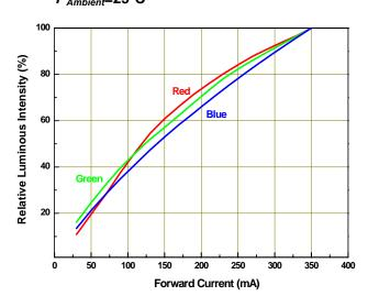
Relative Luminous Intensity vs Forward Current,  $T_{Ambient}$ =25°C
