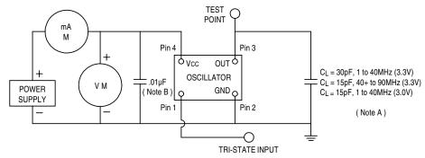
NOTE: A. CL includes probe and fixture capacitance. NOTE: B. An external .01µF bypass capacitor close to package ground and V<sub>CC</sub> pin is required
