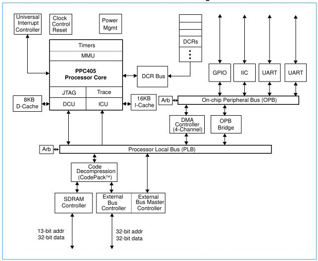
The PPC405CR is designed using the IBM Microelectronics Blue Logic<sup>®</sup> methodology in which major functional blocks are integrated together to create an application-specific ASIC product. This approach provides a consistent way to create complex ASICs using IBM CoreConnect<sup>™</sup> Bus Architecture.
