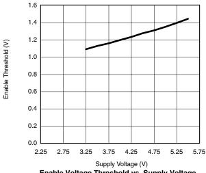
Enable Voltage Threshold vs. Supply Voltage
