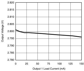
Output Voltage vs. Load Current-Output 1
