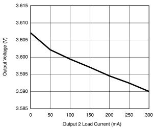
Output Voltage vs. Load Current-Output 2
