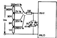
For multi-range, use, a 2 pole, 4 way rotary switch. 1 pole for range select and the other to connect the appropriate decimal point to V+
