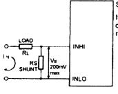
Shunt resistance  $Rs = \frac{Vs}{lin} \Omega$
