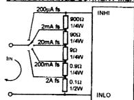
For multi-range, use, a 2 pole, 5 way rotary switch. 1 pole for range select and the other to connect the appropriate decimal point to V+
