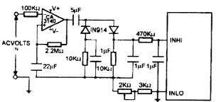
The meter can only measure DC. Use the above circuit to convert AC to DC. For voltages above 200mV AC, a potential divider is required before the converter circuit as shown in the "Voltage measurement" section above
