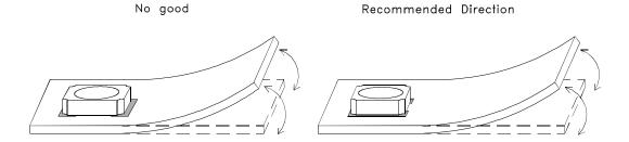
Appropriate LED mounting is to place perpendicularly against the stress affected side.
