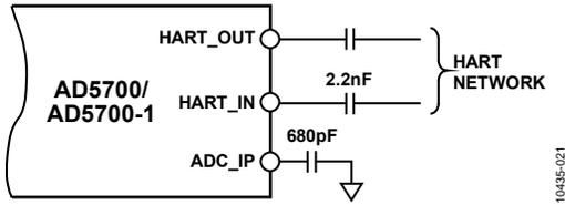
Figure 22. AD5700/AD5700-1 Using Internal Filter on HART\_IN
