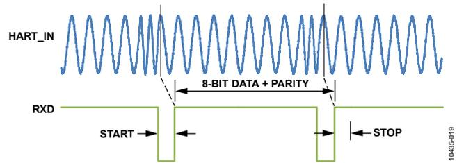
Figure 20. AD5700/AD5700-1 Demodulator Waveform (Preamble Message 0xFF)
