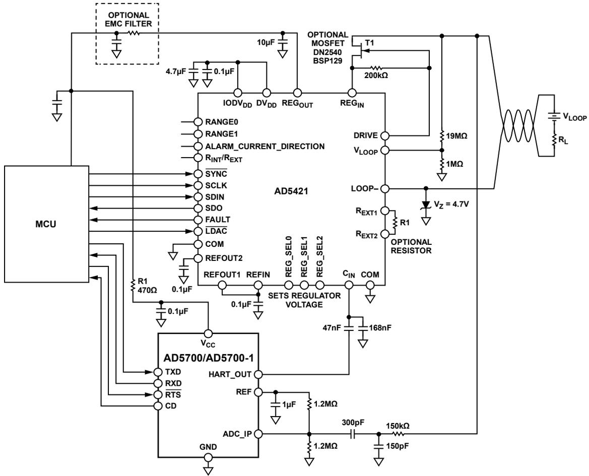
Figure 27. Loop-Powered Transmitter Diagram
