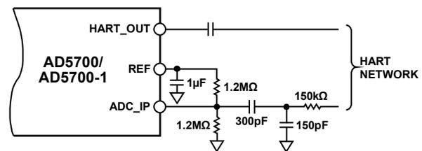
Figure 21. AD5700/AD5700-1 with External Filter on ADC\_IP
