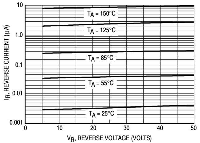
**Figure 3. Leakage Current**
