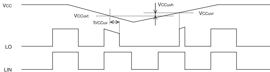
When Vcc Supply Voltage keeps lower UV Trip Voltage ( $VCCuvt = VCCuvt - VCCuvh$ ) for Vcc Supply UV Filter Time, output signal becomes "L". And then, when Vcc Supply Voltage is higher than UV Reset Voltage, input signal (LIN) is L; output signal HO becomes "H".
