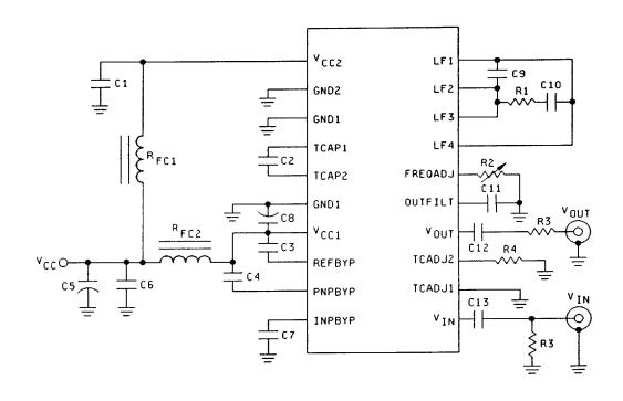
$c_{1}$ ,  $c_{3}$ ,  $c_{4}$ ,  $c_{6}$ ,  $c_{7}$ ,  $c_{8}$ ,  $c_{12}$ , and  $c_{13}$  = 100 nF.  $c_{2}$  = 18 nF (see note 1).  $c_{2}$  = 16 nF (see note 2).  $c_5 = 6.8 \ \mu F$ .  $c_9$  and  $c_{11} = 47 \ p F$ .  $c_{10} = 560 \ p F$ .  $R_1 = 27 \Omega$ ,  $R_2 = 2 \ k \Omega$ ,  $R_3 = 43 \Omega$  (see note 3),  $\rm R_4$  = 3.9 k $\Omega$  (see note 4), and  $\rm R_5$  = 3.9 k $\Omega$  (see note 3). RFC1 and RFC2 = 10  $\mu\rm H.$
