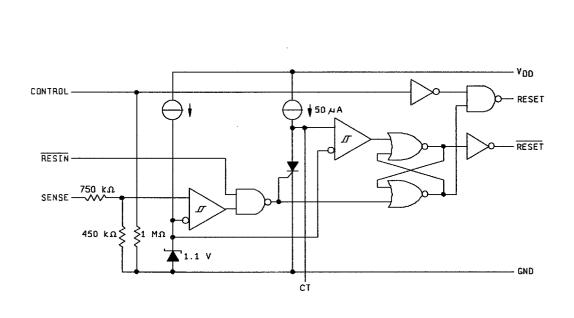
NOTE: Outputs are totem pole configuration. External pull up or pull down resistors are not required.
