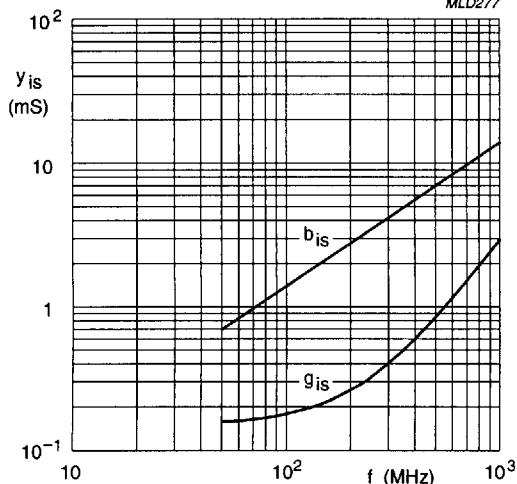
$V_{DS} = 5$  V;  $V_{G2} = 4$  V.
