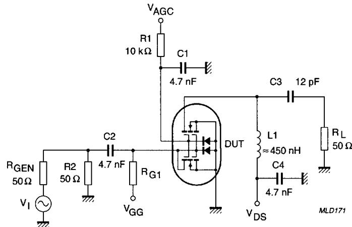
Fig.19 Cross-modulation test set-up.
