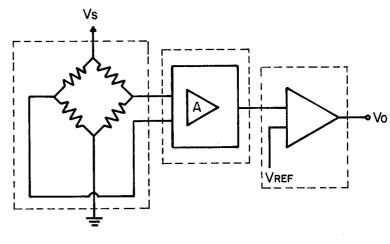
**PIEZORESISTIVE** SENSING **ELEMENT**
