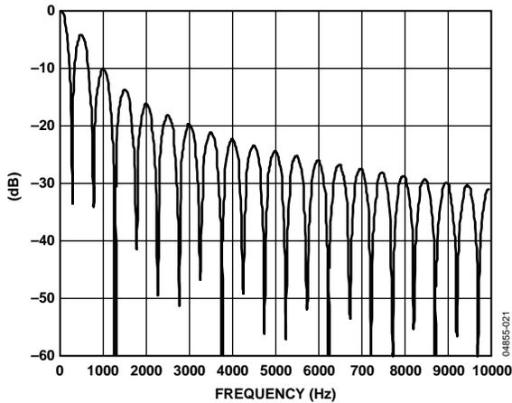
Figure 16. Filter Response at 500 Hz Update Rate
