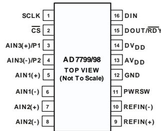
Figure 5. Pin Configuration
