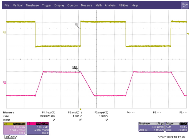
Figure 12. Inverting Large Signal Step Response
