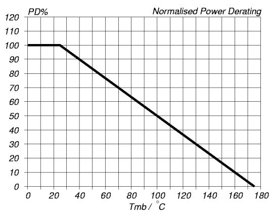
Fig.1. Normalised power dissipation.
