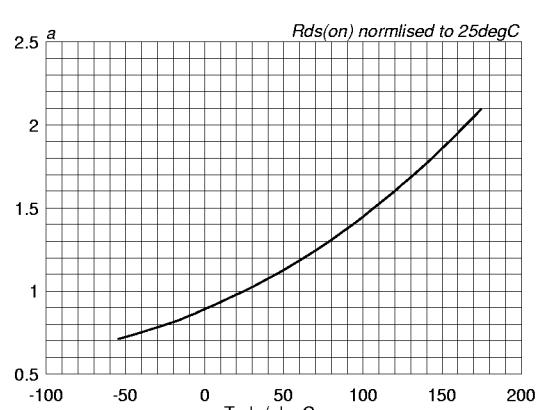
Fig.9. Normalised drain-source on-state resistance.
