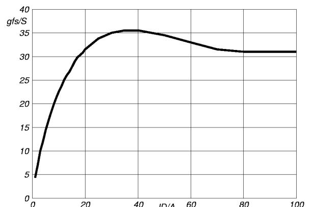
Fig.8. Typical transconductance,  $T_j = 25^\circ\text{C}$ .
