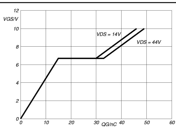
Fig.13. Typical turn-on gate-charge characteristics.
