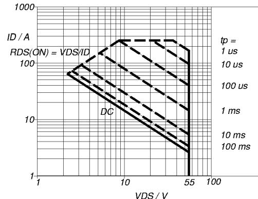
Fig.3. Safe operating area.  $T_{mb} = 25 \text{ }^\circ\text{C}$
