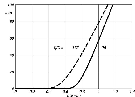
Fig.14. Typical reverse diode current.
