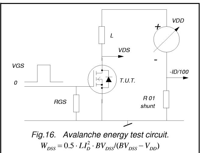
Fig.16. Avalanche energy test circuit.
