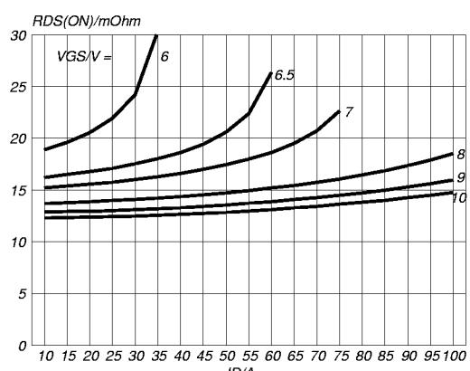
Fig.6. Typical on-state resistance,  $T_j = 25^\circ\text{C}$ .
