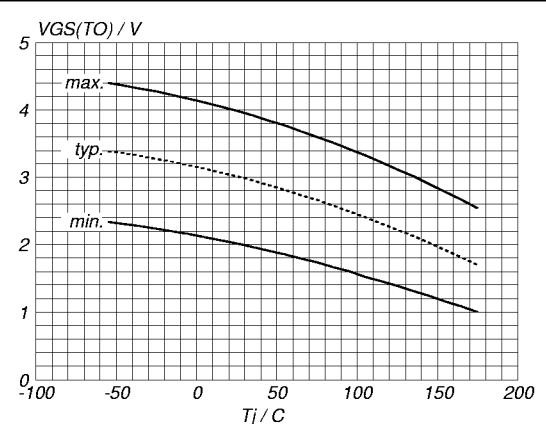
Fig.10. Gate threshold voltage.
