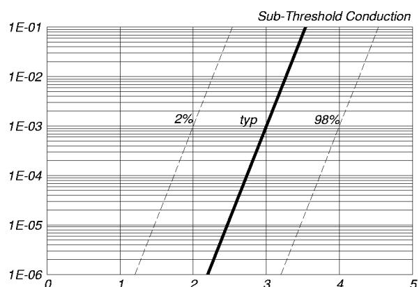
Fig.11. Sub-threshold drain current.
