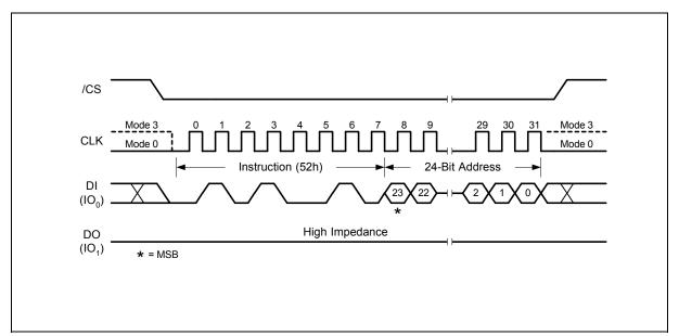
Figure 16. 32KB Block Erase Instruction Sequence Diagram
