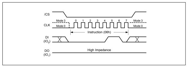
Figure 4. Write Enable Instruction Sequence Diagram
