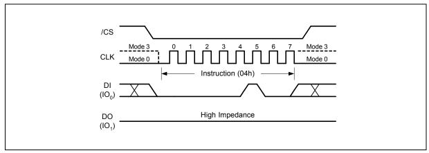
Figure 6. Write Disable Instruction Sequence Diagram
