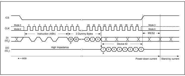
Figure 21. Release Power-down / Device ID Instruction Sequence Diagram
