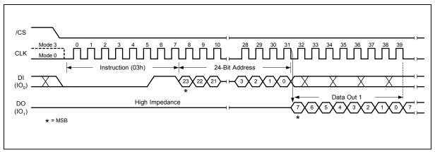
Figure 9. Read Data Instruction Sequence Diagram
