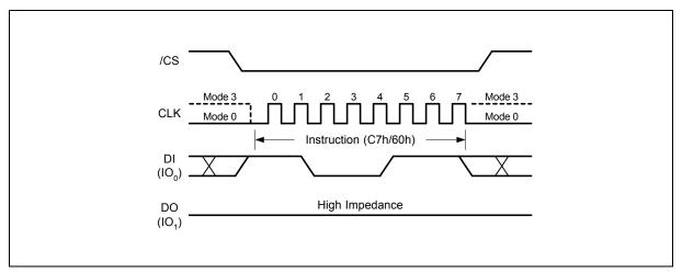
Figure 18. Chip Erase Instruction Sequence Diagram
