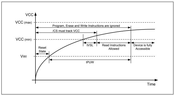
Figure 26. Power-up Timing and Voltage Levels
