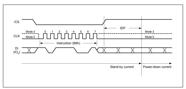
Figure 19. Deep Power-down Instruction Sequence Diagram
