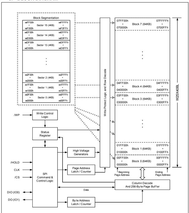
Figure 2. W25X40BL Block Diagram
