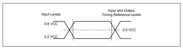
Figure 27. AC Measurement I/O Waveform
