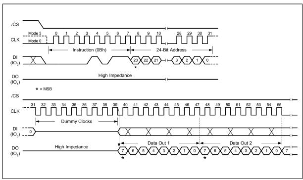
Figure 10. Fast Read Instruction Sequence Diagram
