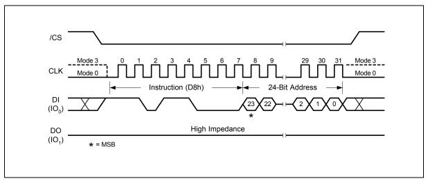
Figure 17. Block Erase Instruction Sequence Diagram
