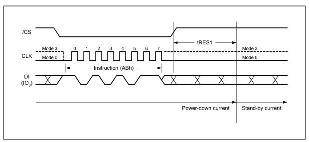
Figure 20. Release Power-down Instruction Sequence
