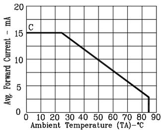
Fig5. MAX. AVERAGE FORWARD CURRENT VS. AMBIENT TEMPERATURE.
