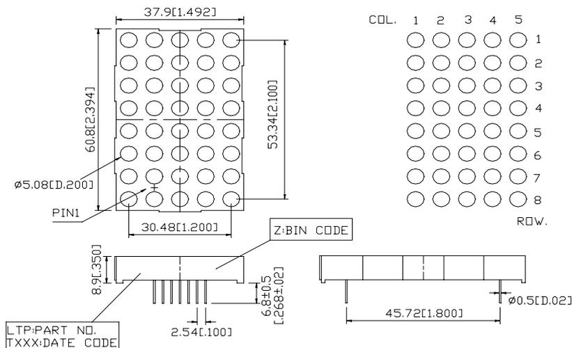
NOTES: All dimensions are in millimeters. Tolerance is  $\pm 0.25$  mm (0.01") unless otherwise noted.
