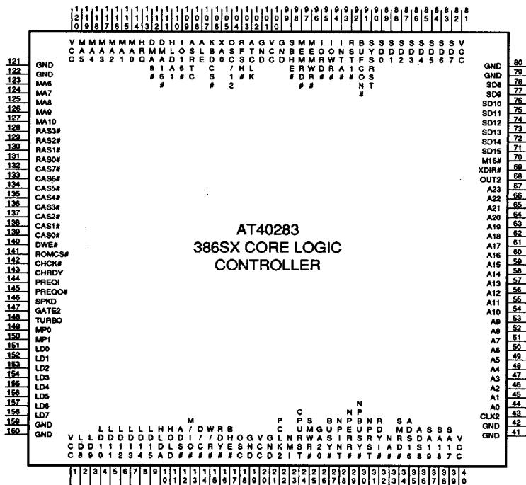
**Core Logic Controller Block Diagram**
