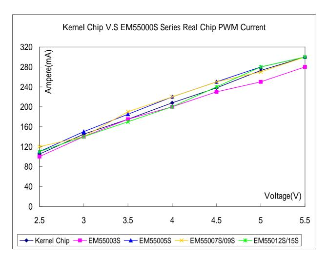
The EM55000S series real chip PWM current only has a very little difference with kernel chip as verified in the above chart.
