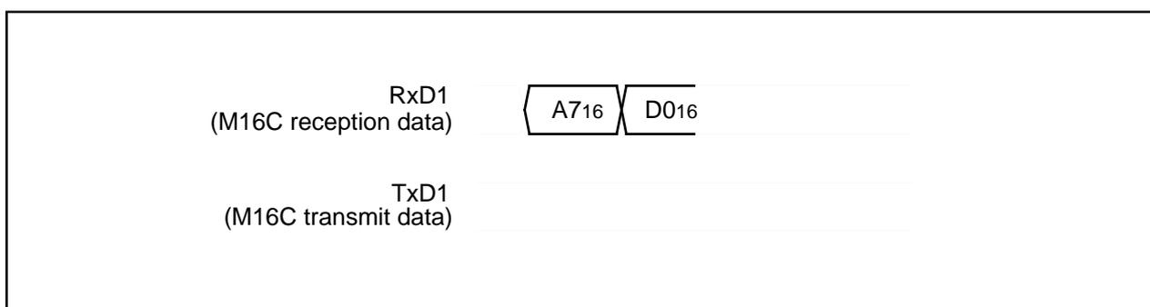
Figure 1.31.29. Timing for erasing all unlocked blocks
