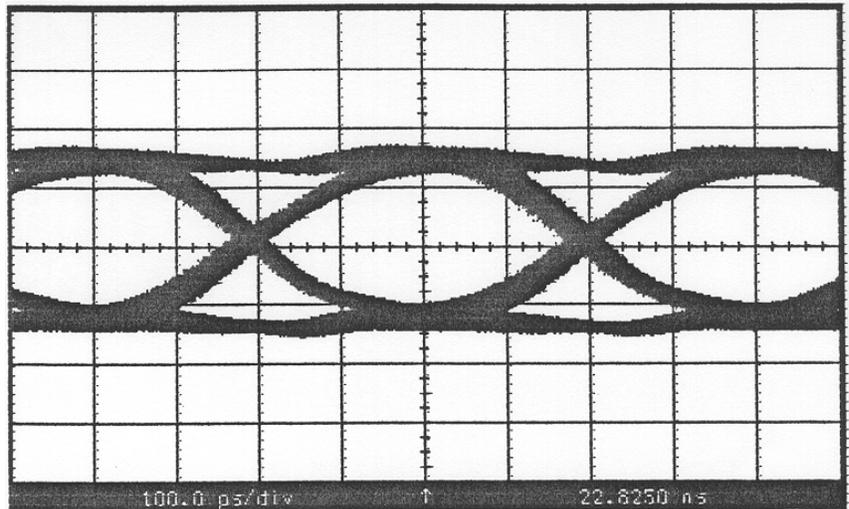
Figure 10. Typical Receiver DATA Output 2488 Mb/s.
