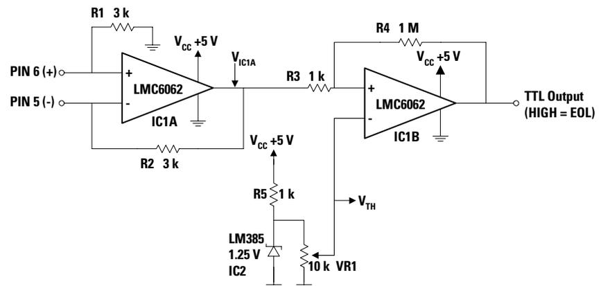
Figure 6. Laser Bias Indicator Circuit
