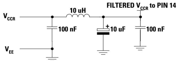
Figure 16. Filter Network for Power Supply Noise Reduction
