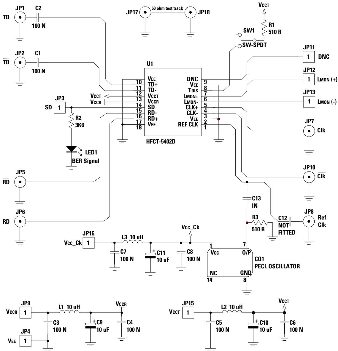
Figure 20. Circuit Schematic for the Evaluation Board
