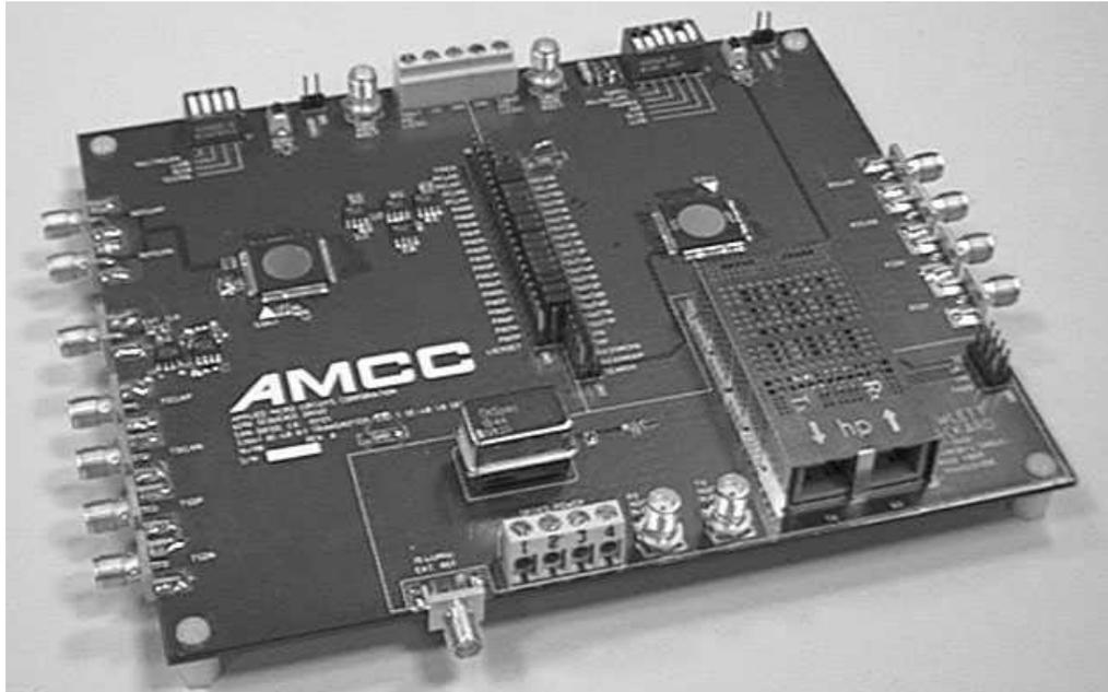
**Figure 22. Reference Design Board**
