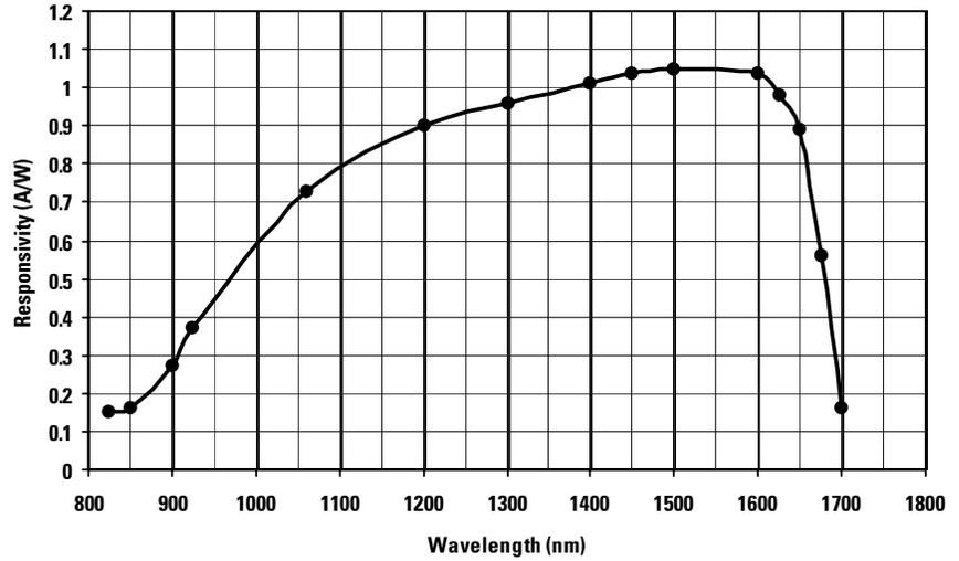
Figure 15. Typical dc Responsivity of an InGaAs PIN Photodiode
