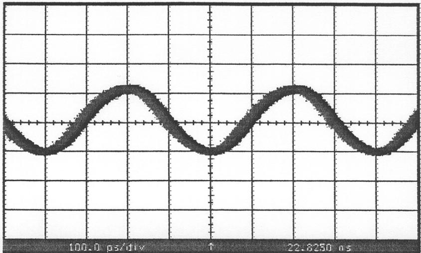
Figure 11. Typical Receiver CLOCK Output 2488 MHz.
