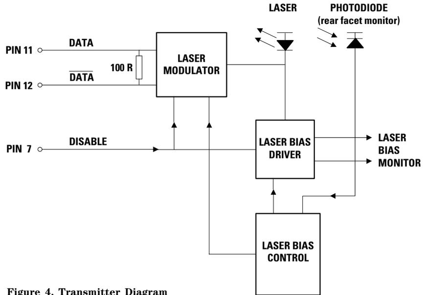
Figure 4. Transmitter Diagram
