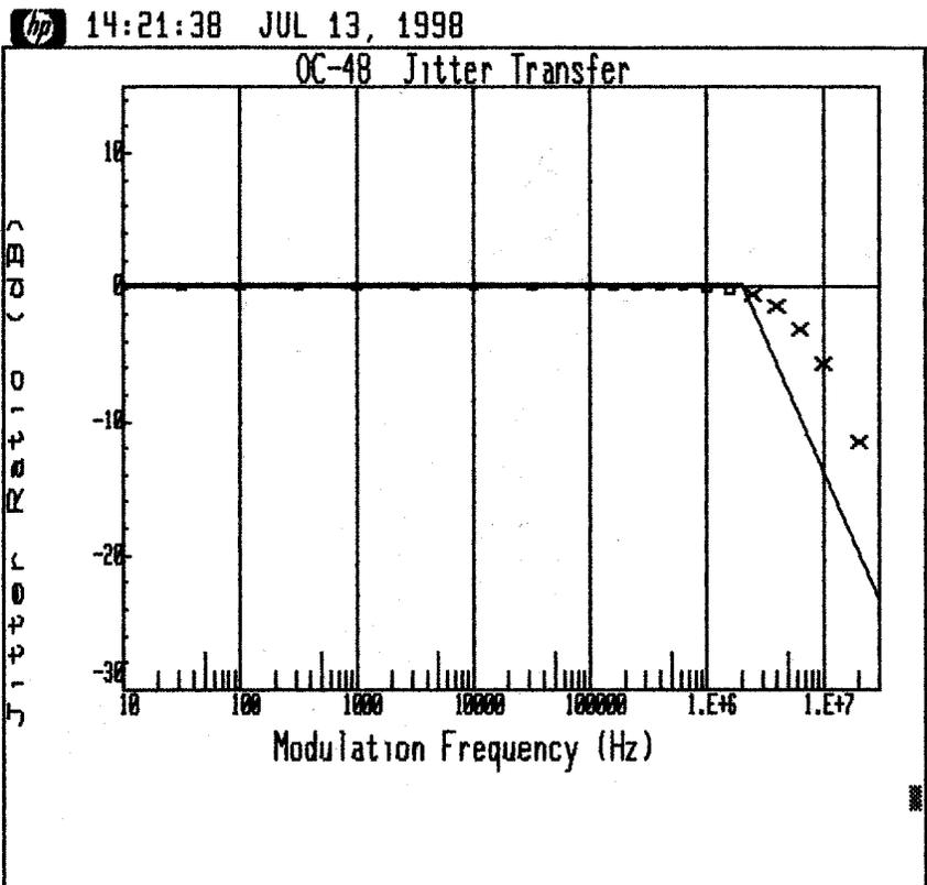
Figure 14. Typical Receiver Jitter Transfer
