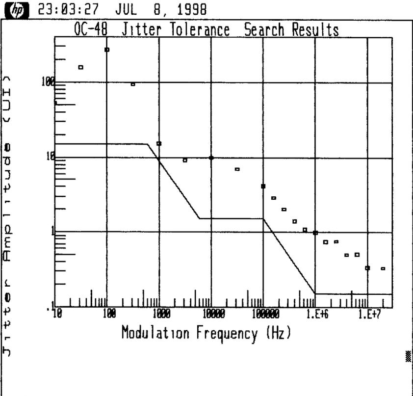
Figure 13. Typical Receiver Jitter Tolerance
