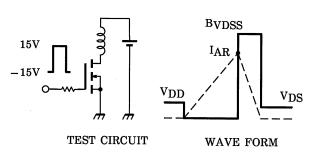
$$\begin{aligned} R_G &= 25~\Omega \\ V_{DD} &= 90~V,~L = 22.9~mH \end{aligned} \qquad E_{AS} &= \frac{1}{2} \cdot L \cdot I^2 \cdot \left( \frac{BVDSS}{BVDSS - VDD} \right) \end{aligned}$$
