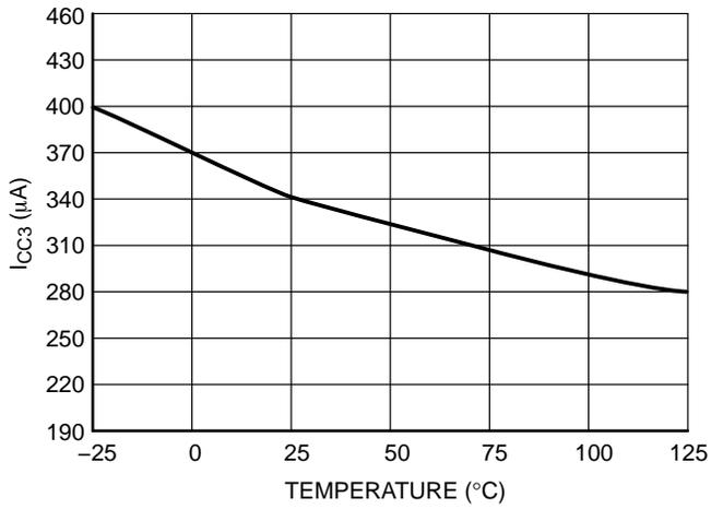
Figure 10. I<sub>CC3</sub> vs. Temperature
