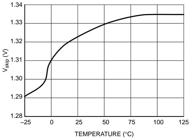
Figure 13. V<sub>skip</sub> vs. Temperature
