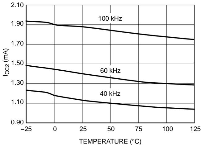
**Figure 7. I<sub>CC2</sub> vs. Temperature**
