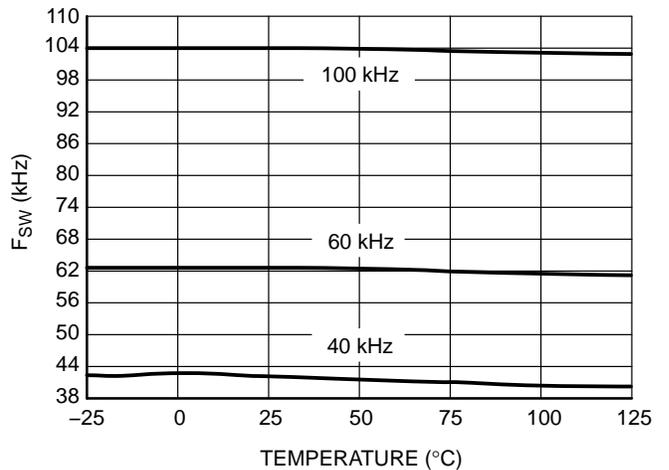
**Figure 8. Switching Frequency vs. T<sub>J</sub>**
