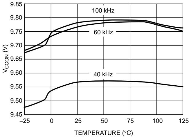
**Figure 5. V<sub>CC</sub> ON vs. Temperature**
