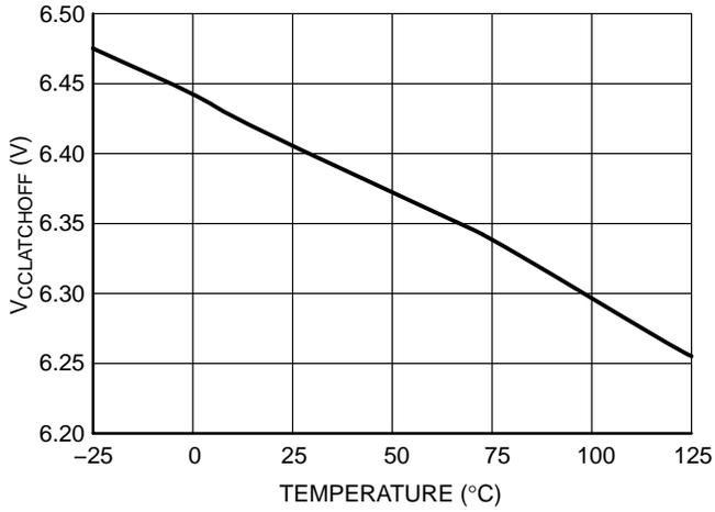
Figure 9. V<sub>CC</sub> Latchoff vs. Temperature
