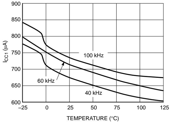
**Figure 6. I<sub>CC1</sub> vs. Temperature**
