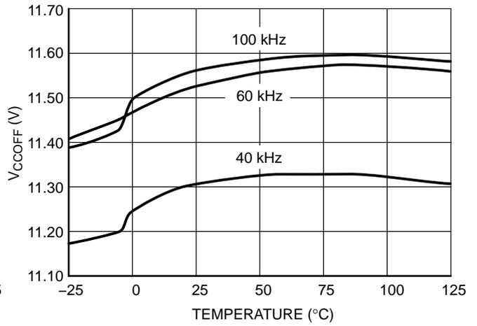
**Figure 4. V<sub>CC</sub> OFF vs. Temperature**
