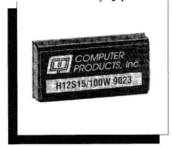
The H Series of low-power PC-mountable DC/DC converters provide premium performance and reliable operation at economical prices. The units provide 1 watt of total output power. All models are encapsulated in miniature 1.0  $\times$  2.0  $\times$  0.38 inch metal cases that provide EMI/RFI protection plus easy installation where space is limited. The H Series is available in 5VDC output models with line and load regulation within 1.0%.
