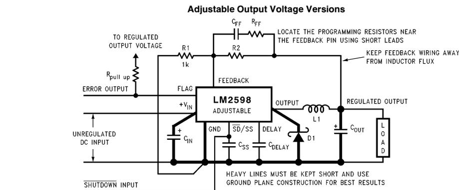
$$V_{OUT} = V_{REF} \left( 1 + \frac{R_2}{R_1} \right) \quad \text{where } V_{REF} = 1.23V$$
