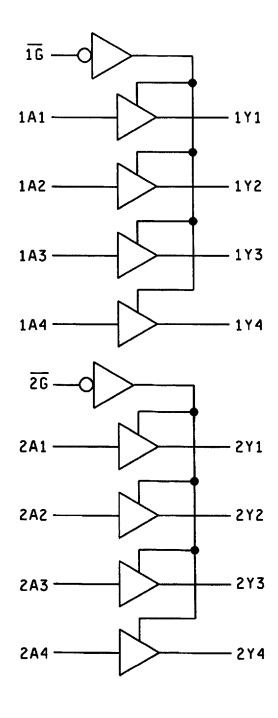
FIGURE 3. Logic diagram.
