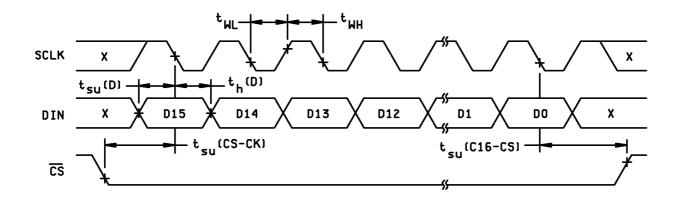
FIGURE 3. Timing waveforms.
