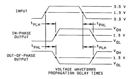
NOTES: 1. C<sub>L</sub> includes probe and jig capacitance.
