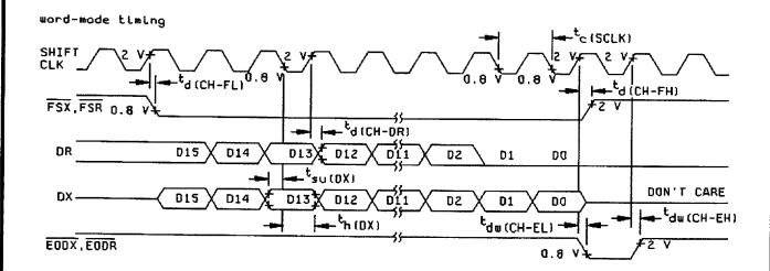
FIGURE 5. Serial port timing waveforms.
