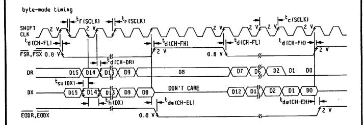
FIGURE 5. Serial port timing waveforms - Continued.
