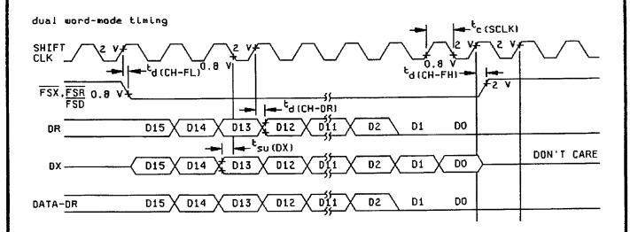
FIGURE 5. <u>Serial port timing waveforms</u> - Continued.
