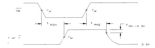
Three-state output enable time to low level and output disable time from low level
