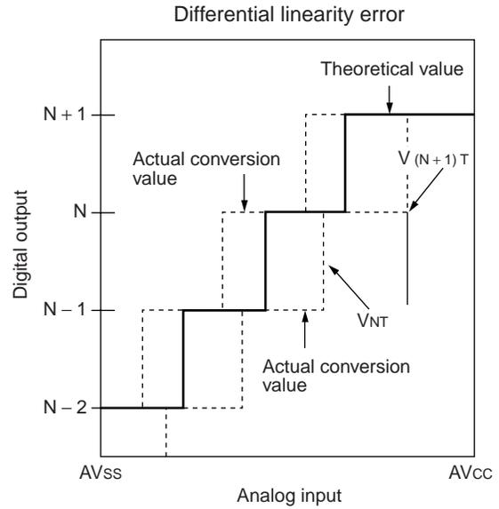
$$\text{Differential linearity error} = \frac{V_{(N+1)T} - V_{NT}}{1 \text{ LSB}} - 1$$
