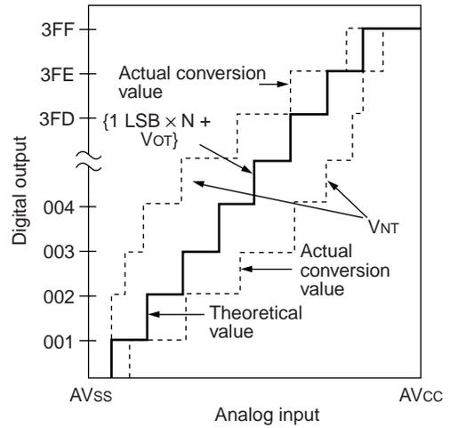
$$\text{Total error} = \frac{V_{NT} - \{1 \text{ LSB} \times N + 0.5 \text{ LSB}\}}{1 \text{ LSB}}$$
