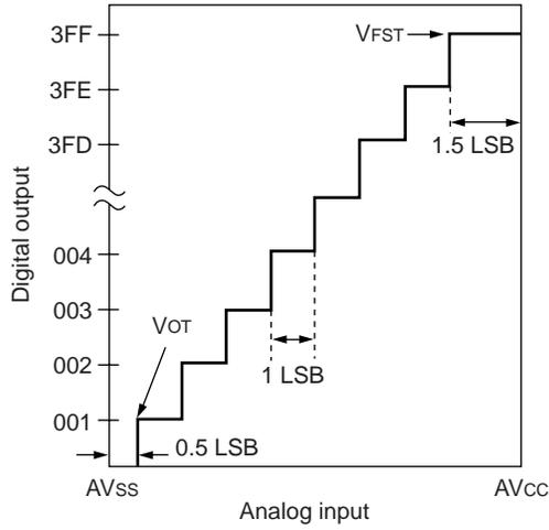
$$1 \text{ LSB} = \frac{V_{FST} - V_{OT}}{1022} \text{ (V)}$$
