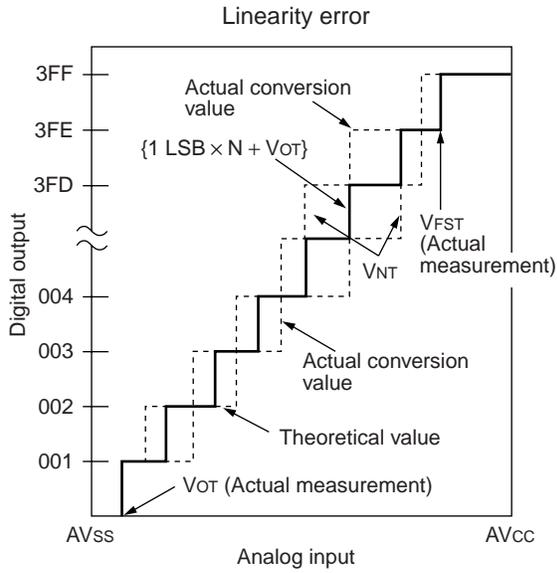
$$\text{Linearity error} = \frac{V_{NT} - \{1 \text{ LSB} \times N + V_{OT}\}}{1 \text{ LSB}}$$
